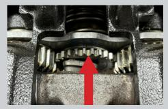
Webb heavy-duty NH225 and LN225 calipers are equipped with a robust centralized gear-driven adjuster, offering enhanced reliability and durability.
